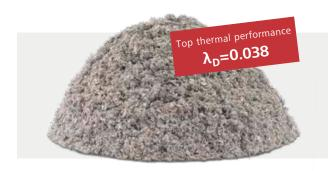
Only sorted daily newspaper is used for STEICOfloc. This is defibred in a modern vortex mill. A low proportion of inorganic mineral salts ensures the material's lasting durability and fire protection.
